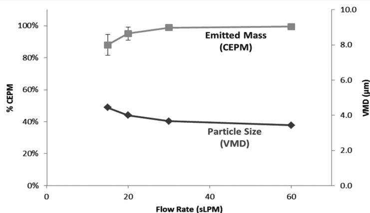
Figure 2. Dispersibility properties of lead IgG iSPERSE formulation across flow rates in terms of emitted mass from capsule and particle size, n=5 (lot G). The formulation had an IgG loading of greater than 25% and showed good stability by SDS-PAGE and IEF.
